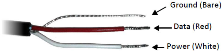
Figure 2: Pigtail End Wiring
