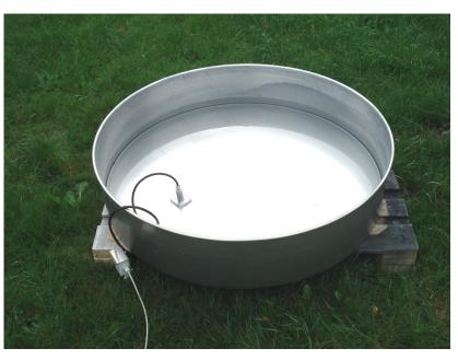
The Evaporation Gauge ET10 is a high accuracy pressure transducer designed to measure water depths of around 250 mm for use in a standard Evaporation Pan CLASS A Pan. The sensor is very precise and can be upgraded in most existing mechanic CLASS A Pans. The pan is manufactured in corrosion resistant aluminium. For siting and location of the pan WMO recommendations (publication WMO No.8 'Guide to Meteorological Instruments and Methods of Observation'. Sixth edition, 1996) should be
