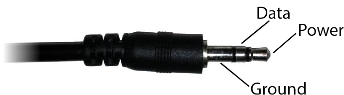
Figure 5: 3.5 mm Stereo Plug Wiring
