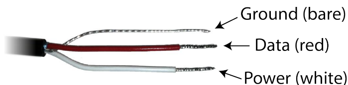
Figure 6: Pigtail End Wiring
