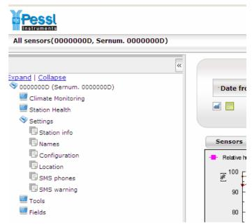
enter the logging interval, the time zone, the transmission times and an telephone number to which an emergency SMS is send on malfunction of the iMETOS. "Location" offers you a tool to enter the GPS position of the iMETOS by the use of maps or satellite pictures. The links "SMS phones" and "SMS warning" are needed to set up an alert system for frost or soil moisture.
